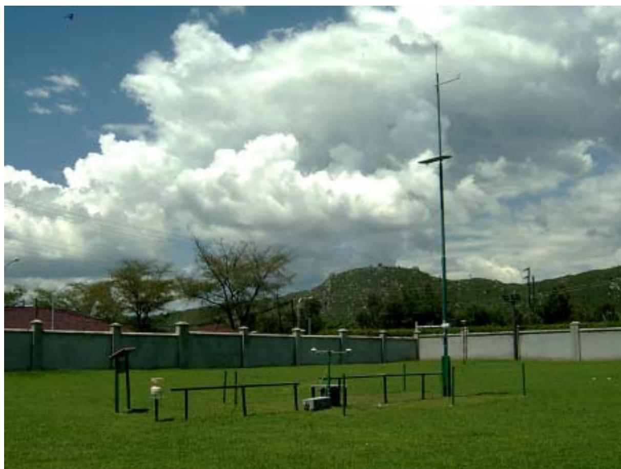
Figure 1.4 Automated weather stations at KEMRI, measuring radiation, air temperature, relative humidity, wind speed and rainfall.
